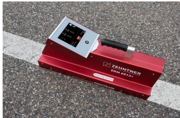
Figure 2. Measurement process using Zehntner ZRM 6013+ RL/Qd retroreflectometer on "Babur" street.
