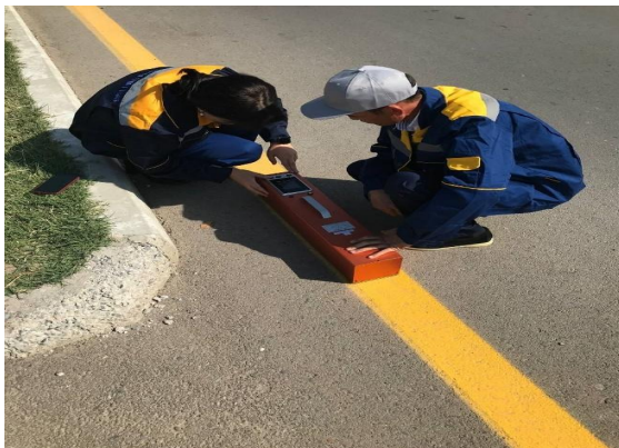
Figure 2. Measurement process using Zehntner ZRM 6013+ RL/Qd retroreflectometer on "Babur" street.
