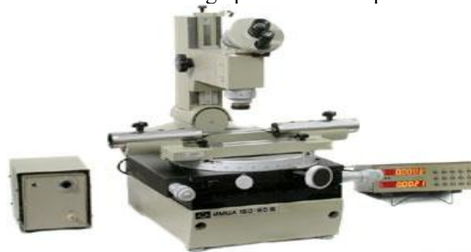
Figure-8. IMTS 150x50B (BMI-1TS) brand instrument microscope is used for measuring chisels, mills, grinders and other tools.
