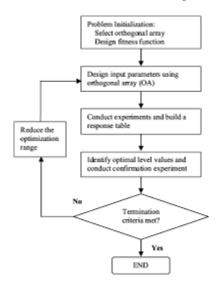
Experiments were conducted using state-of-the-art LBW equipment, precisely controlling the selected parameters as per the Taguchi design matrix. Welds were produced under various combinations of parameter settings, allowing for the generation of a robust dataset that covered a wide spectrum of welding conditions. The quality of each weld was rigorously evaluated, considering factors such as weld bead geometry, porosity, and heat-affected zone (HAZ) characteristics.
