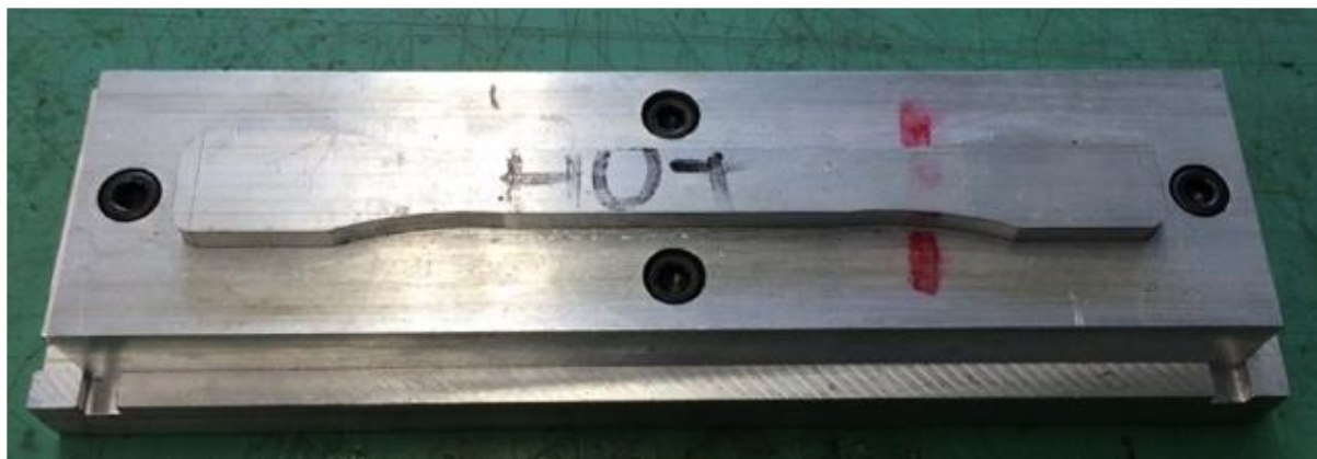
Figure 14. ASTM D638 Aluminum mold
