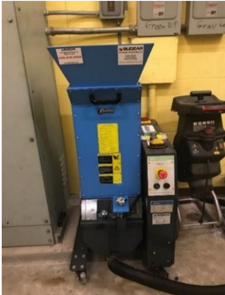
Figure 13. Heavy Duty shredder used to make small granules.
