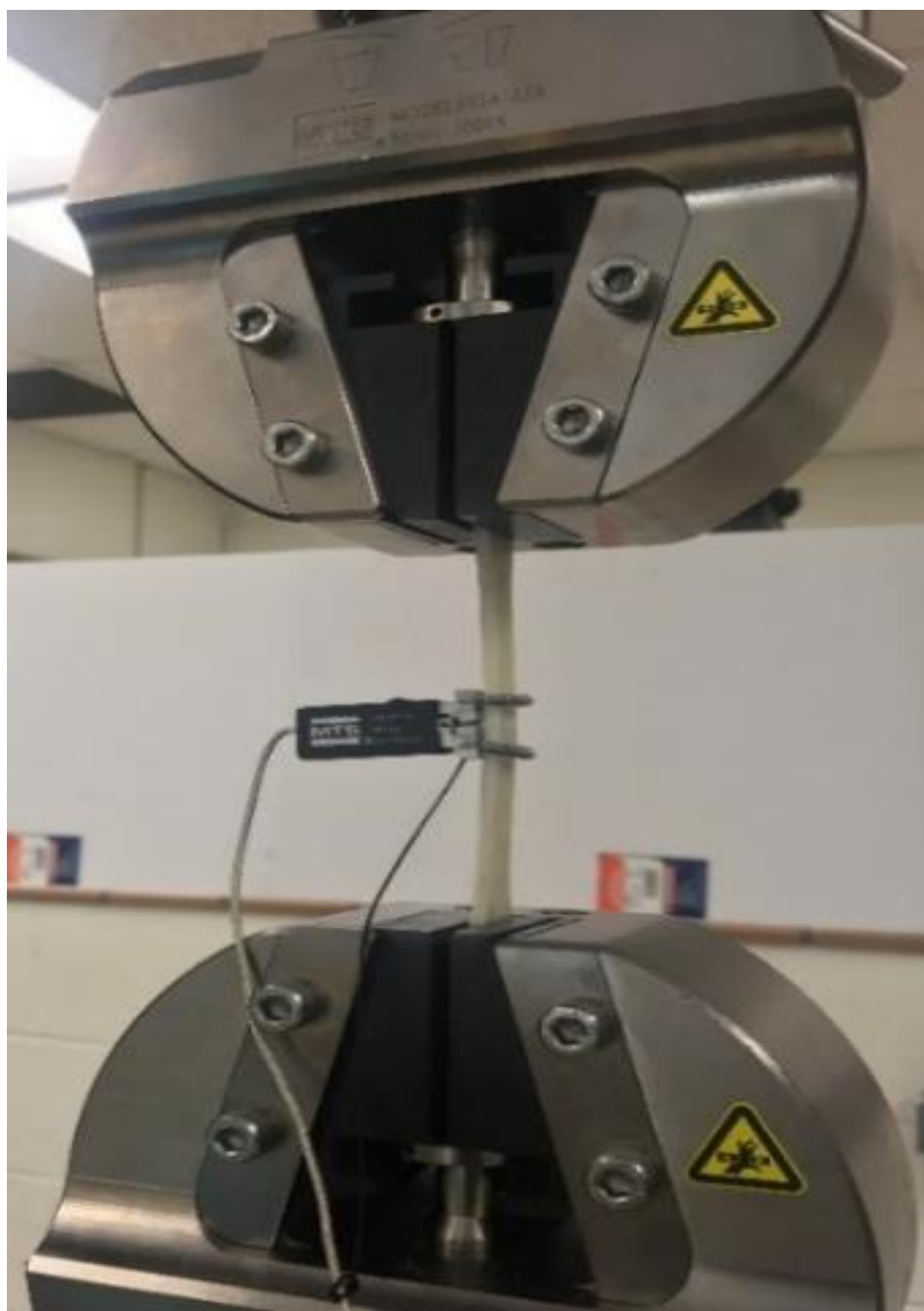
Figure 17. MTS Grips and Extensometer setup.
