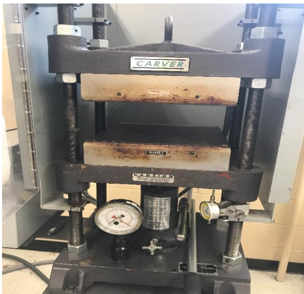
Figure 15. Heated press for compression molding.
