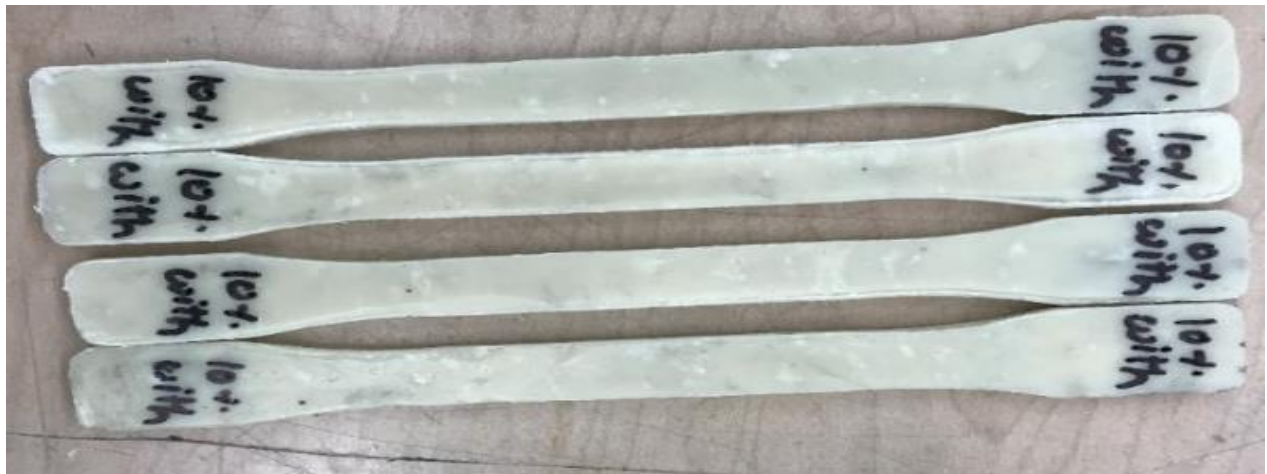
Figure 16. Thermoplastic specimens from an ASTM D638 mold using compression molding.
