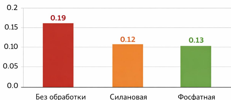
Figure 2. Corrosion rate depending on fiber treatment
