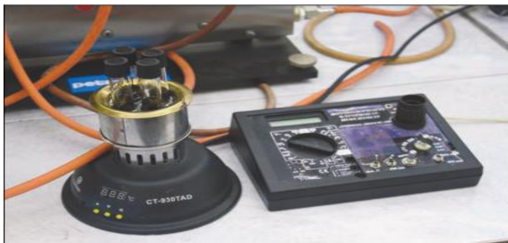
Image 3. Device for determining the thermal stability of diesel fuel samples (left - a steam or water bath for heating samples, right - "Unifot" photometer for determining the optical density of combustion).
